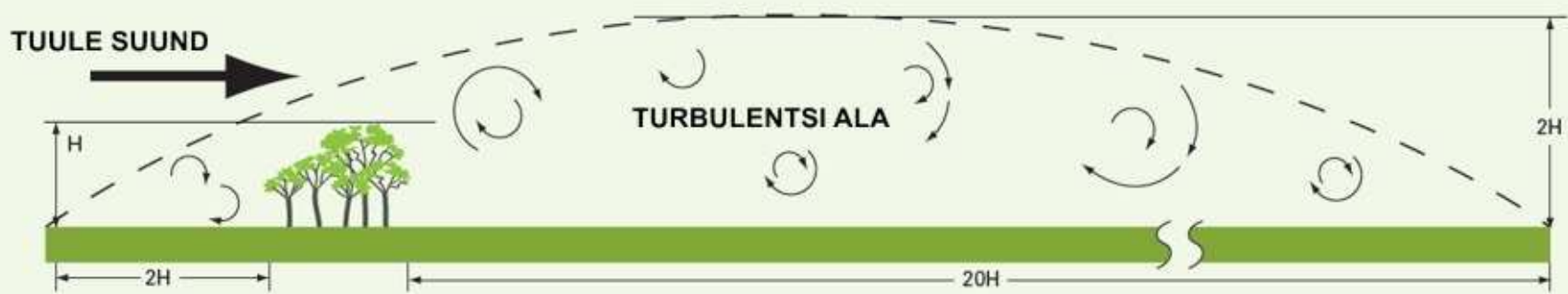
Figure 2.3: Turbulence 'shadow' cast by obstacle
