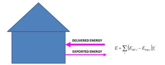
System boundary for nearly net zero energy building definition, connecting a building to energy networks. Net delivered energy is delivered  $E_{\rm del,i}$  minus exported energy  $E_{\rm exp,i}$  accounted separately for each energy carrier i. Primary energy E is calculated with primary energy factors  $f_{\rm i}$  as shown in the figure.
