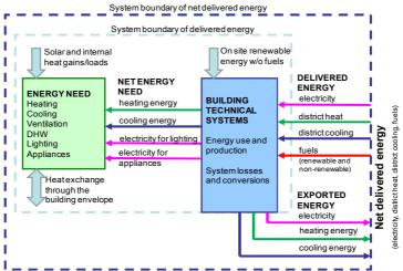
Energy boundary of net delivered energy. The box of "Energy need" refers to rooms in a building and both system boundary lines may be interpreted as the building site boundary.
